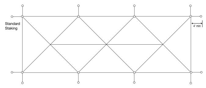
Note: Additional stakes will be necessary in soft soil conditions or whenever stakes pull up from the ground.
