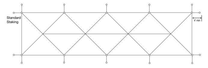
Note: Additional stakes will be necessary in soft soil conditions or whenever stakes pull up from the ground.
