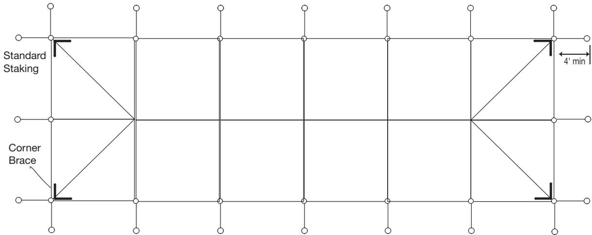
Note: Additional stakes will be necessary in soft soil conditions or whenever stakes pull up from the ground.
